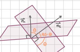
The angle between z planes is found through finding the angle between their norms, this is equivalent due to complementary angles.
